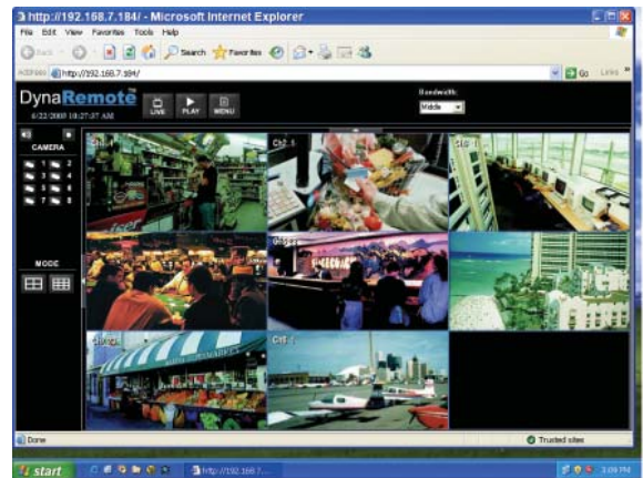
The DynaRemote™ software allows users to remotely monitor, record, playback, archive, change system settings, and control dome cameras over internet.
