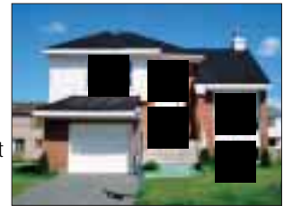
Areas with swaying trees or flickering light, etc. can be eliminated to avoid false alarms. Surveillance of the detected object can be conducted at a zoom magnification of x1.0, x1.4, x2.0 or x2.6.
